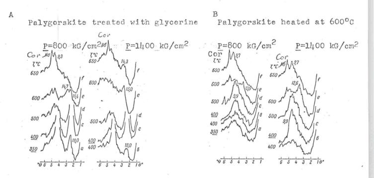
Fig.3. Parts of diffractograms of the phases developed in palygorskite sample at  $\underline{P}_{H_20} = 800$  and  $\underline{1}400 \text{ kG/cm}^2$  and  $\underline{T} = 350$  to  $650^{\circ}\text{C}$ after 22-48 hour runs; <u>A</u> - sample treated with glycerine after experiment; <u>B</u> - sample heated at atmospheric pressure for 2 hours at  $600^{\circ}\text{C}$
